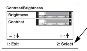
The command line at the bottom of the control screen tells what to do next from this screen. You can toggle between control screens, adjust the selected option, or exit the screen.
